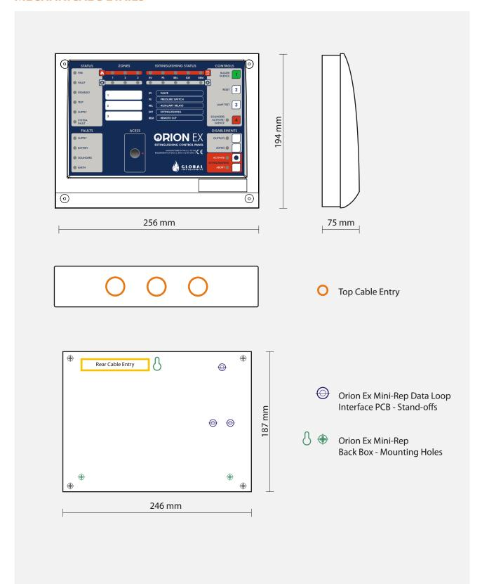
Figure 1: ORION EX MINI-REP - Installation
